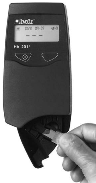
HemoCue haemoglobin meter 201 showing microcuvette in loading position. Courtesy HemoCue AB .
