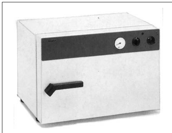
Plate 7.3 WTB Binder E 28 model, 60–230°C hot air oven with external thermometer and timer and fitted with thermostat and overheat cut-out. Courtesy of WTB Binder.
